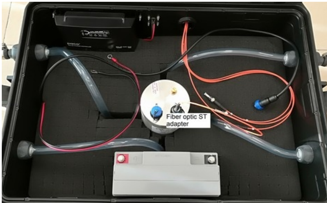
Figure3. Fiber cable connection.
