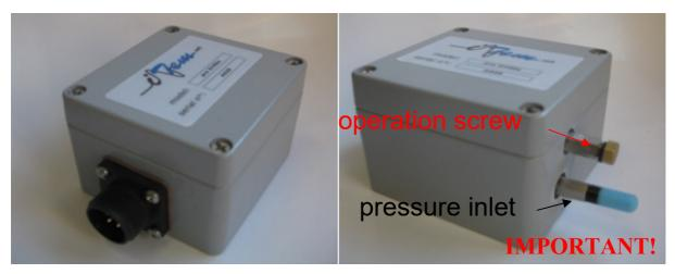
fasten the operation screw before sensor operation
